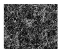
Scales of silicon carbide nanowires (SiC-NWs) were synthesized by thermal evaporation of ferrocene onto silicon wafers at high temperature. The SiC-NWs have diameters of  $\approx 20$  nm and lengths of several  $\mu ms.$  A tentative growth model on the basis of a vapor-liquid-solid (VLS) mechanism was proposed.
